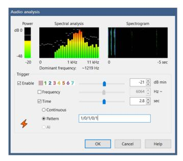
Pattern matching provides methods to specify more complex signal matching. 1's and 0's are used to denote dB power spikes over time. This example shows 3 hand claps within 2.8 seconds and a corresponding trigger.
