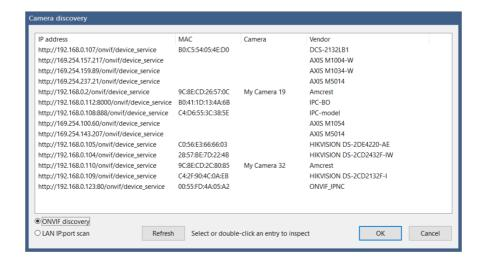
You may instead select **LAN IP:port** scan to examine all IP addresses and then detect common camera ports.
