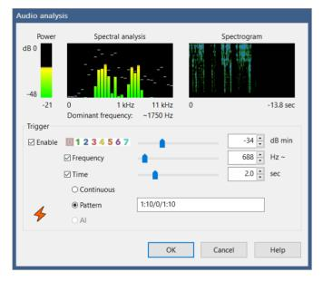
Here, triggering was achieved with a typical human voice speaking range (100-1000 Hz). The pattern shown here requires two instances of approximately 688 Hz over 2.0 seconds with a break between these. Also shown here, the minimum time for the pattern make/break may be overridden for each pattern component (in milliseconds) by placing it after a colon. The future addition of frequency ranges may further the utility of this type of detection.
