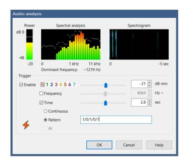
Pattern matching provides methods to specify more complex signal matching. 1's and 0's are used to denote dB power spikes over time. This example shows 3 hand claps within 2.8 seconds and a corresponding trigger.
