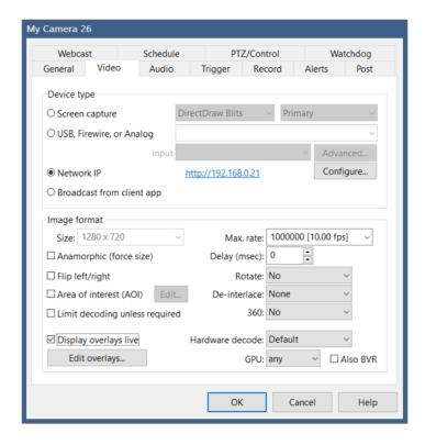
The **Screen capture** device offers a method to use the PC screen as a camera source. You may choose the capture technology, one of:
