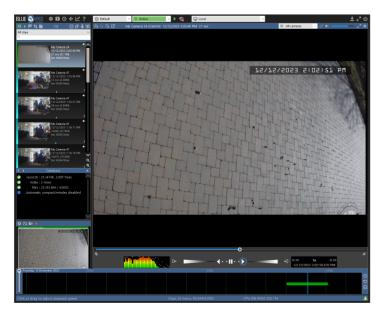
The clip viewer now features audio visualization in the form of spectral analysis. This display is updated as the video moves at any speed, with or without audio played on the speakers. As AI may be applied to spectrograms in the future, this may become an exciting way in which to *search clip audio* for specific types of sounds.
