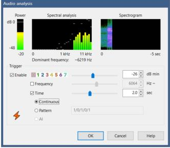
You may specify that the signal must maintain a dB level for a set duration. The signal represented in this example is high frequency white noise.
