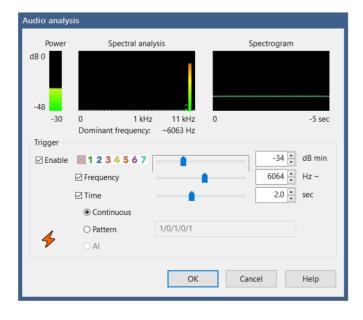
Here a signal generator was used to provide a proper frequency over the required 2.0 seconds in order to trigger. You may use this to recognize your doorbell, phone ringer, fire or other home alarms.
