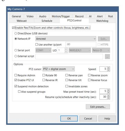
When using a network IP camera, the type of camera has likely already been pre-populated here for you. Rarely for USB cameras, a PTZ interface is exposed through the DirectShow driver and that may be selected here.
