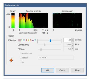
The most basic model involves triggering with a single significant sample set over a specified minimum dB level.
